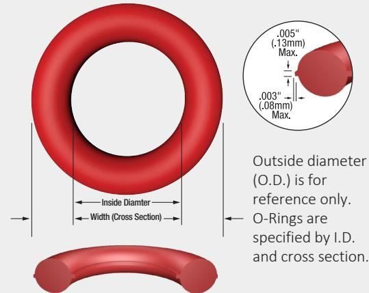
\* Shrinkage Size Adjustment: Various o-ring compounds exhibit different shrinkage rates during molding. The normal o-ring sizes herein shown are based upon a 70 Durometer Nitrile standard. For other o-ring materials, be sure to consult your Apple representative.
