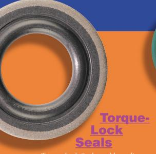
Iorque-Lock Seals enable sealing under the head of a standard fastener, without any special modifications to the fastener or mating parts. A composite seal consisting of an elastomer bonded to a metal washer/retainer, Torque-Lock is ideal for axial applications involving face-type fittings.
