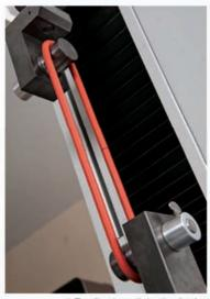
^ Tensile strength testing is also available if necessary
